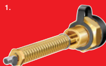
1. Internal tank safety valve (anti-vacuum valve), with plastic protective cap. Internal thread, 1" NPT, external thread, M 48 x 1.5.
